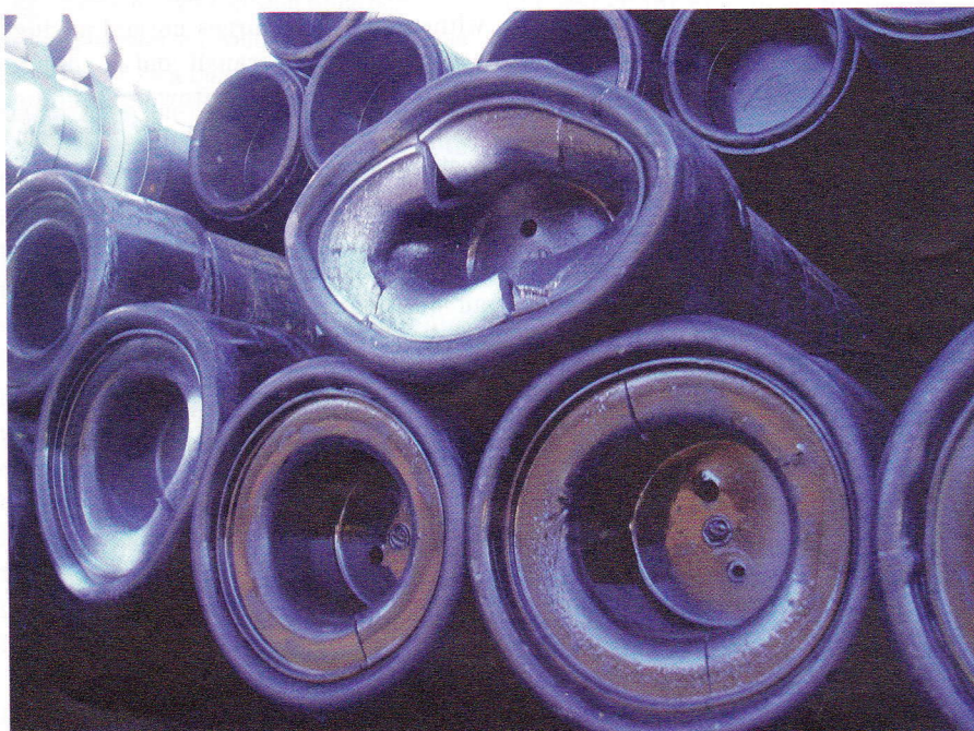
▲ Pipes damaged from compression on the stowage
