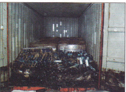
▲ Container of spirits from flooded and oil contaminated cargo hold
