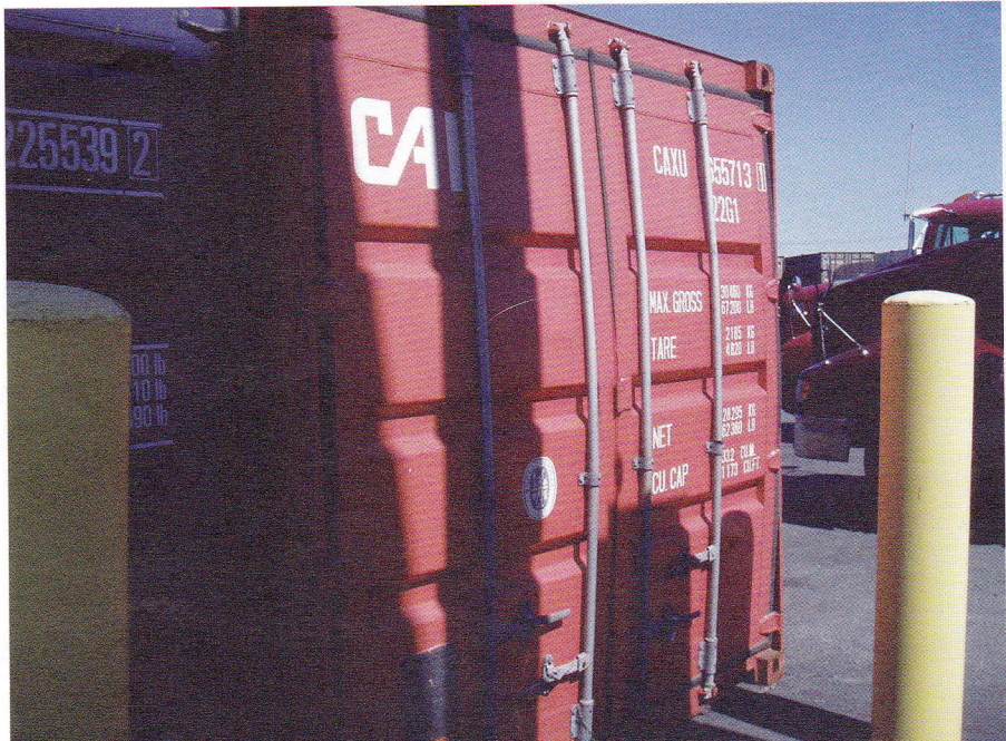
▲ Container with doors bulging, resulting from longitudinal shifting of cargo. Cause: insufficient securing
