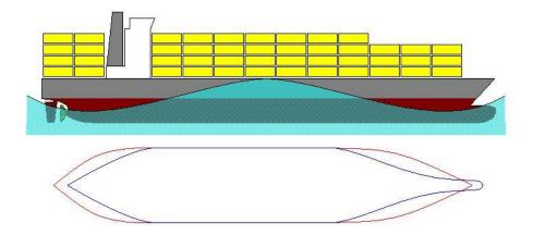
When the trough reaches the midship section, the area of the water plane is maximum, even more so than it would be in calm waters: the midship section is fuller even in low waterplanes, while the crests are at fore and aft end above water level which due to the hull geometry and bow flares have a much larger submerged volume. As result of this increased water plane area, the values of metacentric height (GM) and righting arms (GZ) are increased too.
