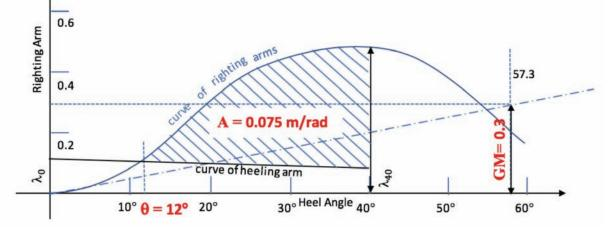
The documentation on board should be complete enough to show that the vessel meets all the intact and grain stability criteria for a specific loading plan (as well as longitudinal strength and hold mass criteria), including:
