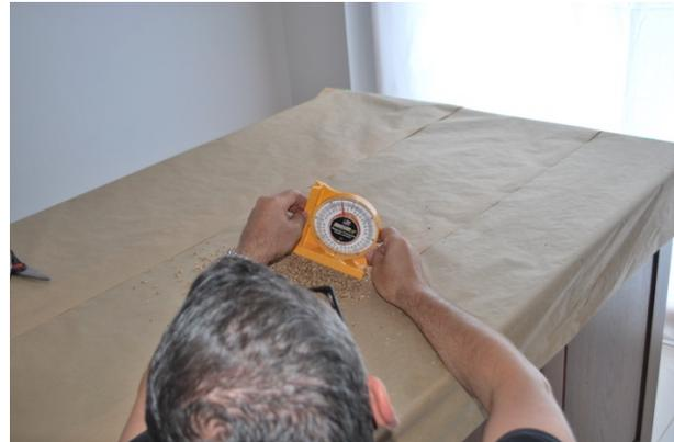
Figure 18: Detail of measurement of AOR taken with the level indicator.
