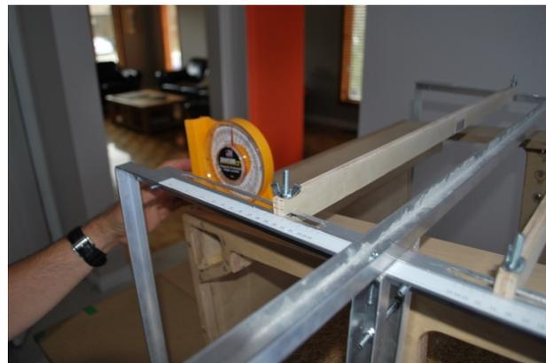
Figure 22: Detail of protractor with reading of the permanent angle of list after the shifting.
