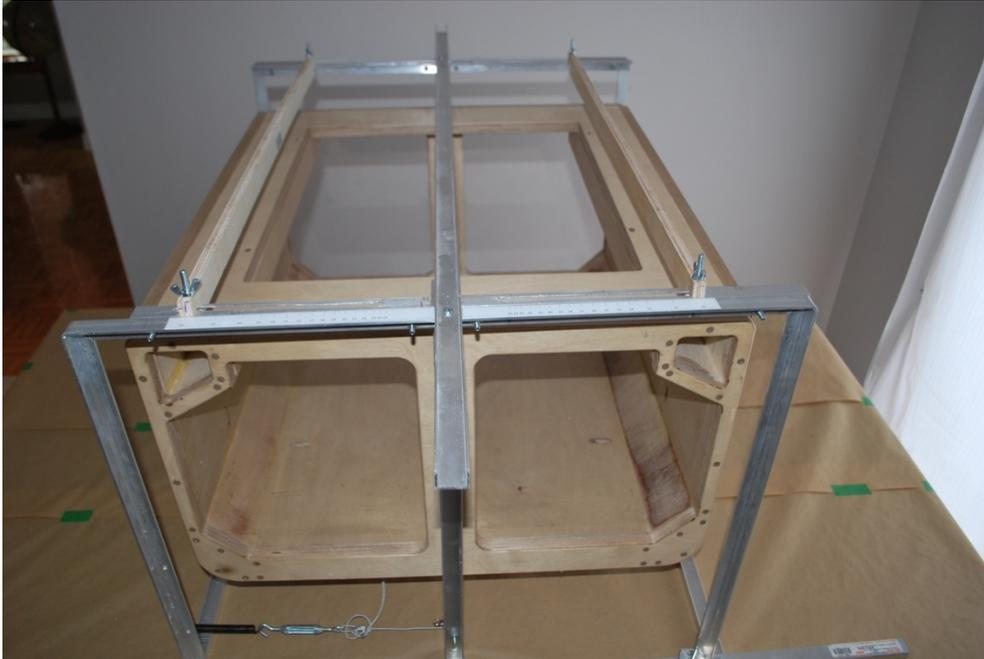
Figure 13: Photograph of the angle limiting mechanism with longitudinal sliding bars and scale.
