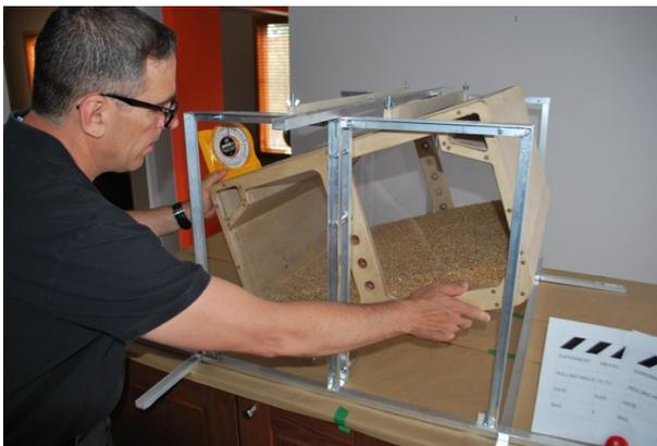
Figure 21: Rolling the model and measuring the AOS, closer view, with fixed axis.
