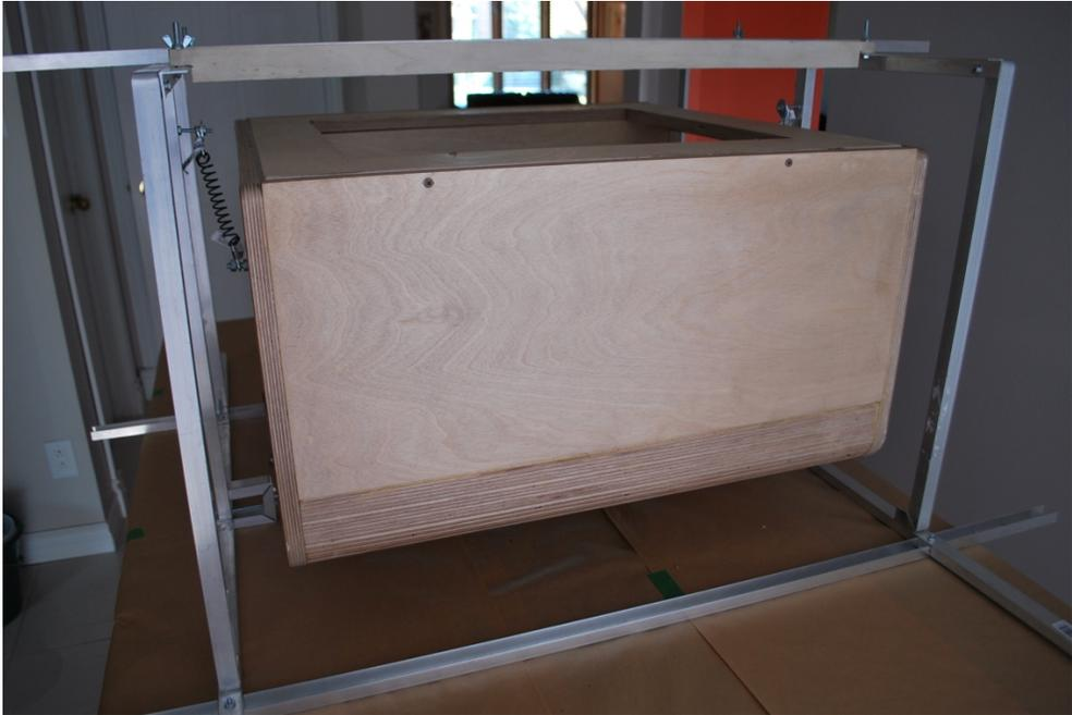
Figure 11: Photograph of the model and support assembly with springs.
