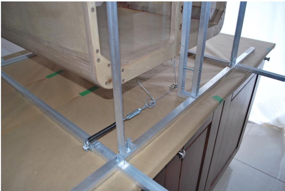
Figure 14: The spring and cable assembly for damped oscillations.
