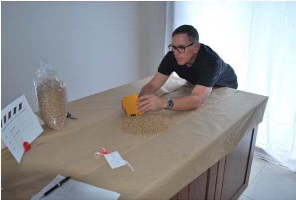
Figure 17: Performing the measurements of AOR with level indicator.
