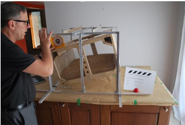
Figure 25: Rolling the model and measuring the AOS, closer view, with springs.
