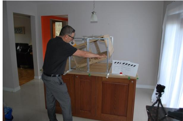
Figure 20: Rolling the model and measuring the AOS, with fixed axis.
