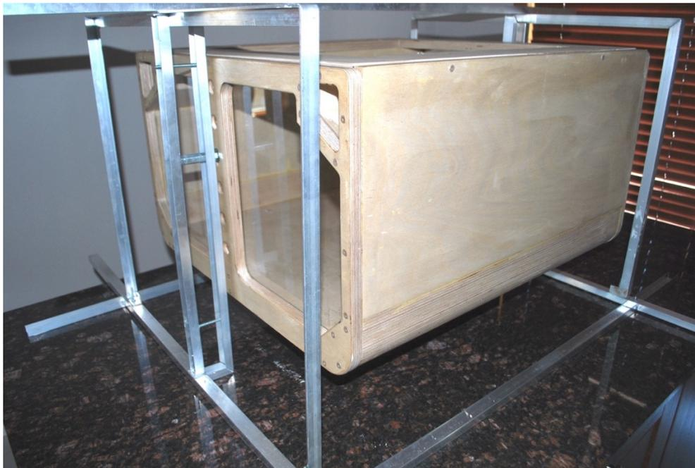
Figure 10: Photograph of the model and support assembly with fixed axis.
